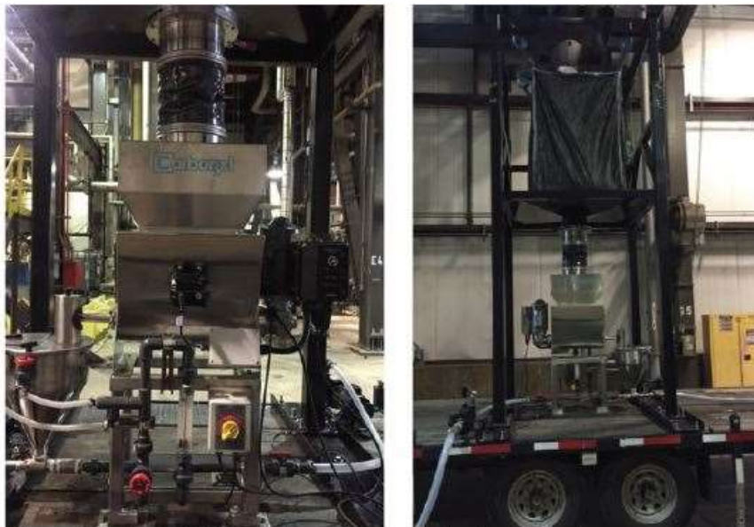
Figure 2. Carbonxt pilot test equipment. The only plant requirements are a source of water, and electricity. Maintenance includes replacing the bag of activated carbon as needed. Typical change out rates are every 1-2 days.
