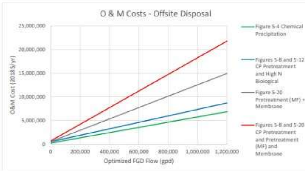
Figure 4-3 Comparison of EPA's O&M cost curves (EPA, 2019a)
