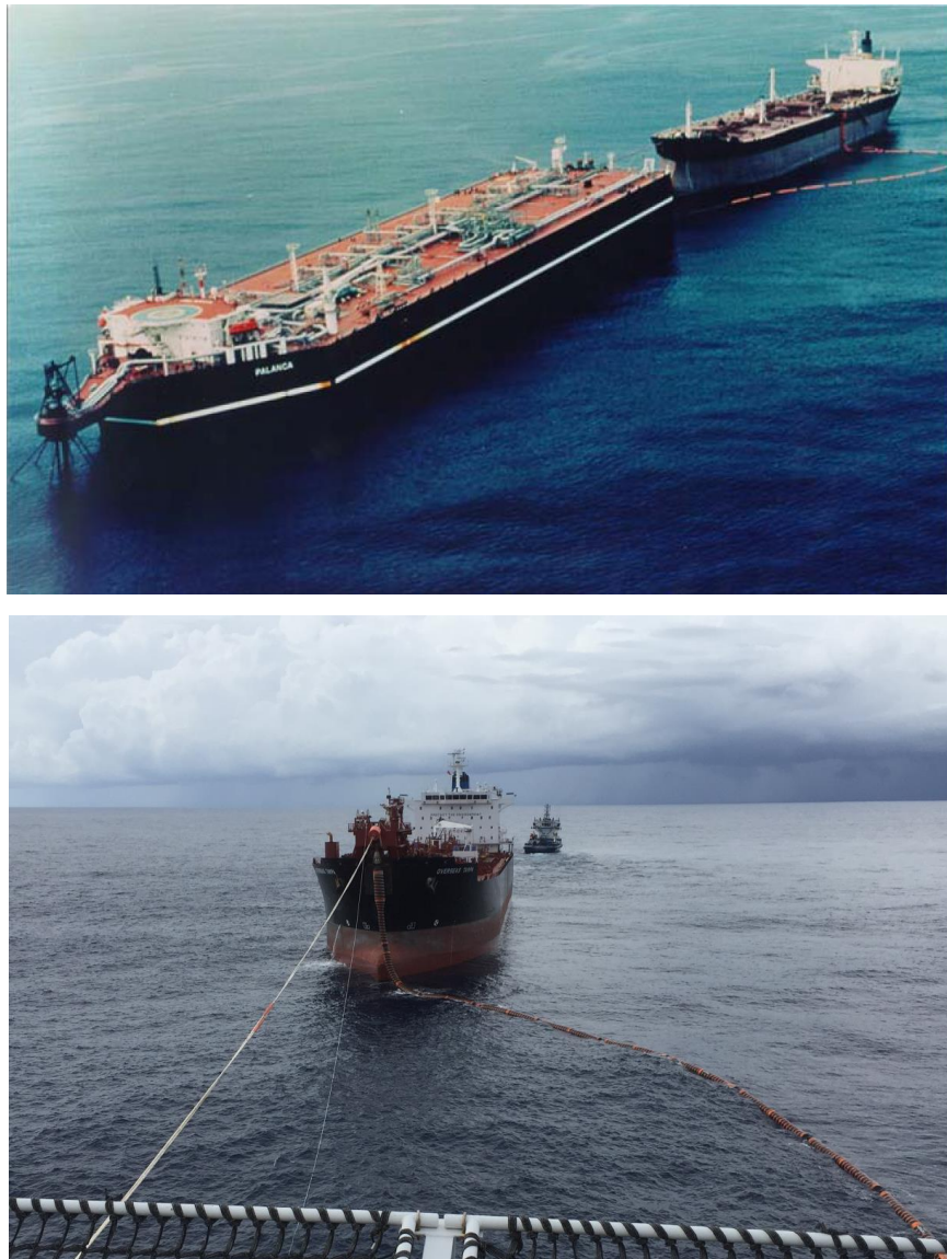
Figure 7-1 Tandem Offloading from F(P)SO to Shuttle Tanker 122,123
